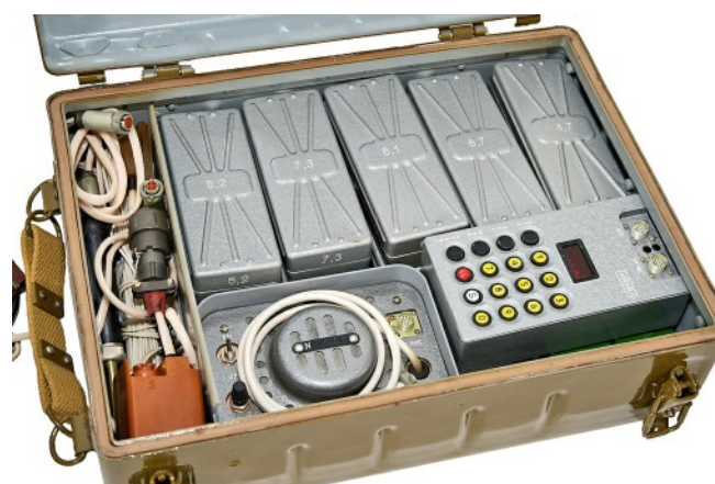
Severok K packed in metal unit transport case. For operational use in the field the loudspeaker and most of the plug-in RF units were not required.
